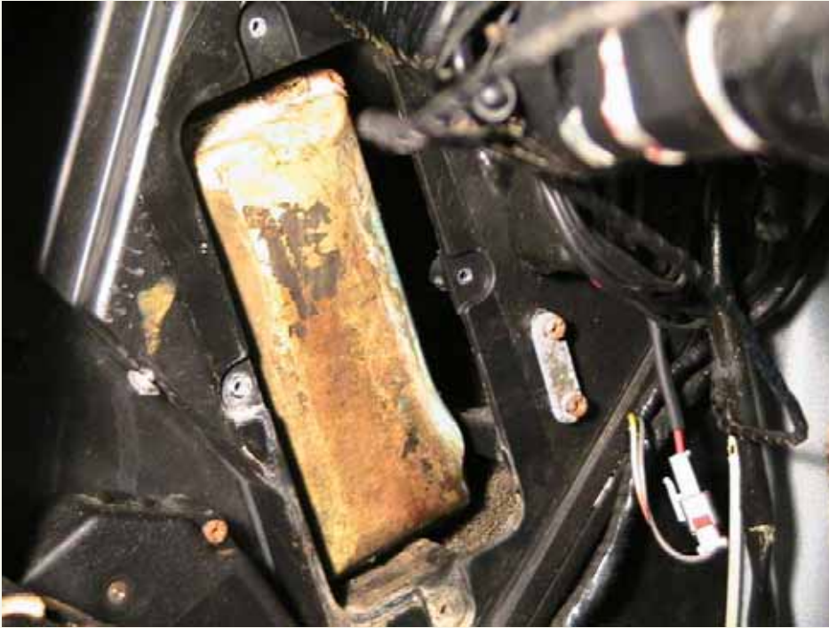
End cover plate removal revealed missing foam seal around heater core.
