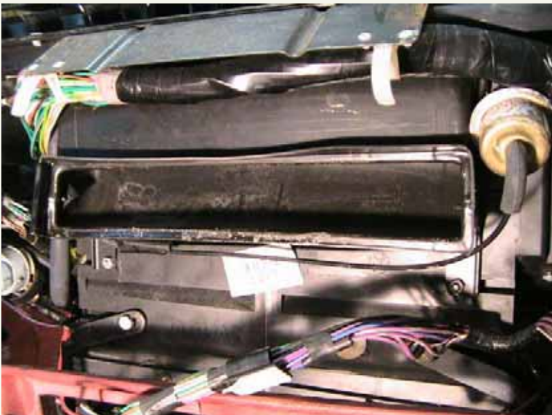
Also, ducting from the AC unit to the center face vent was found to be distorted from 17 years of service, preventing proper engagement of the center face level vent.
