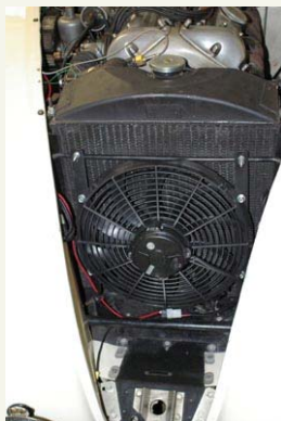
Left— Fan Installation in front of the radiator
