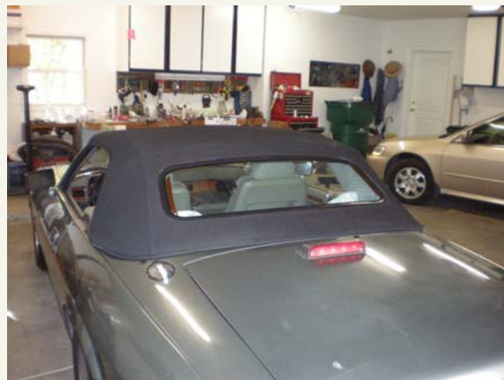
Top and backlight (rear window) installation complete.
