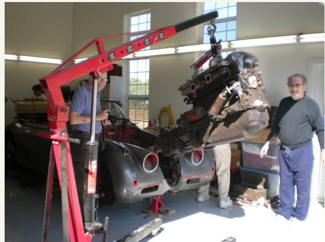
Engine and transmission clear the car.
