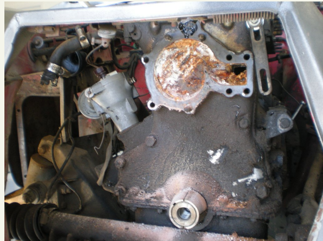
Front of engine with water pump and damper removed.
