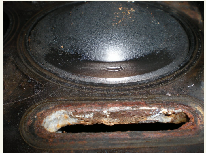
Two pistons showed evidence of intake valve contact.
