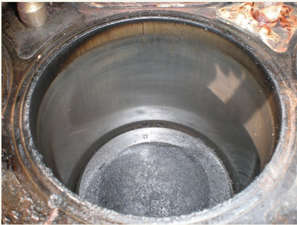
Clean bore without rust, scoring or ridge.
