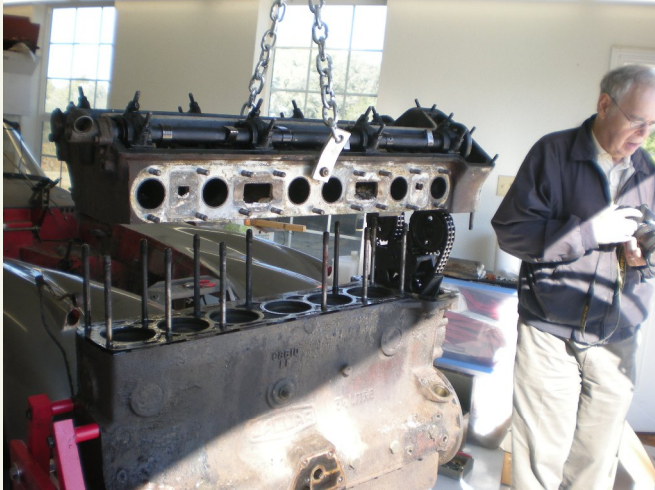
Cylinder head was removed without difficulty.
