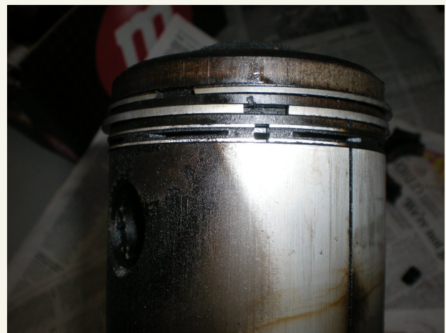
Ring gaps were clustered on most pistons. This allows both oil and compression leakage.
