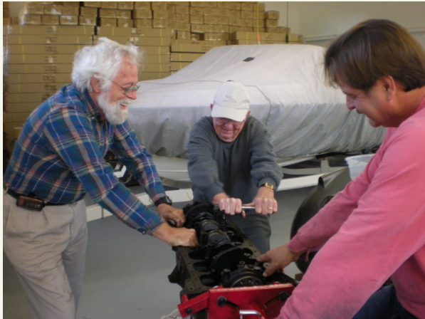
Andy and Richard brace the engine stand while SJC President Bob Olson works to break loose a main bearing bolt.
