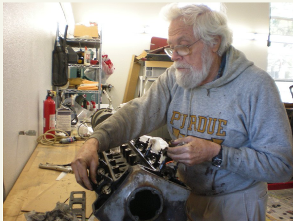
Andy replaces bearing caps after removing camshafts.
