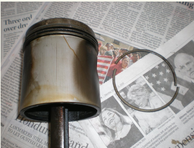
#1 piston had a crack and a broken lower compression ring. A total of five rings were broken.
