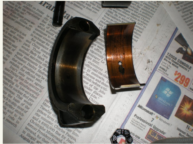
#1 connecting rod lower bearing shell.
