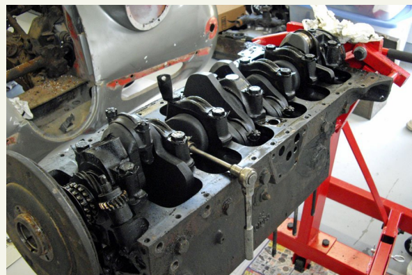
View of the block and crank of the XK engine; to give an idea of size, the ratchet handle in the foreground is about 7" (175 mm) long.
