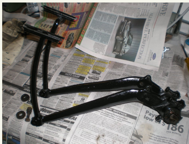
Pedal assembly ready for re-installation.
