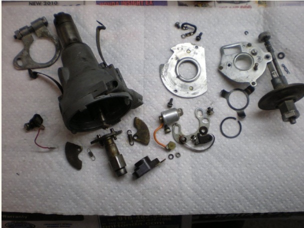
Distributor broken down for cleaning.
