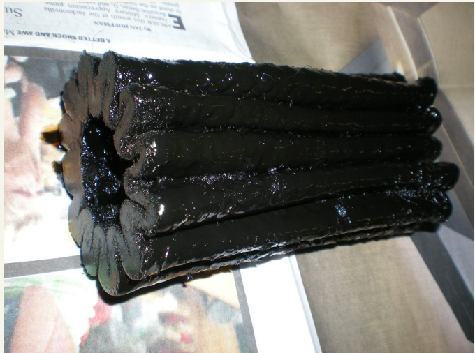
Slightly sludged up filter element.
